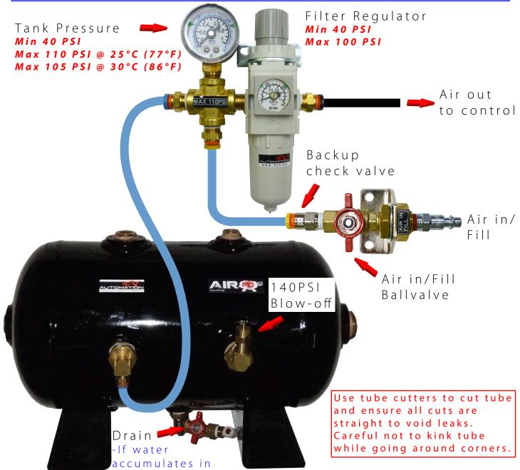
tank slowly open ball valve to drain water.
